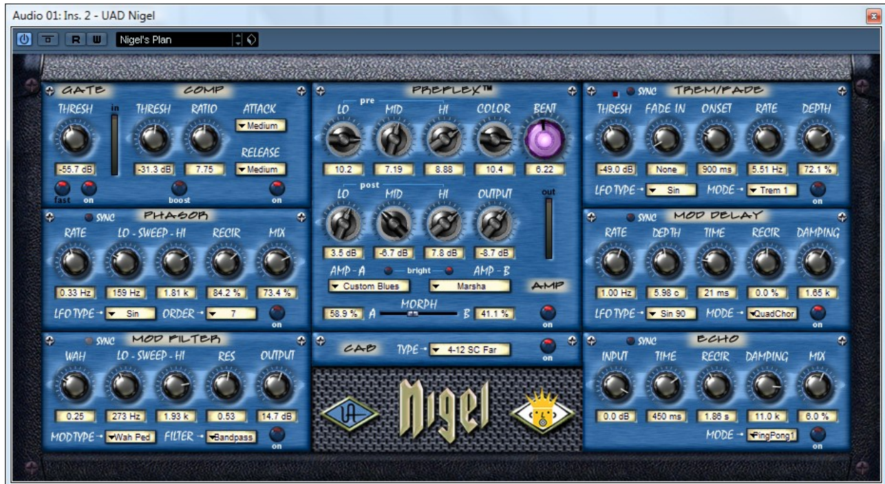
Speaker Simulator including Compressor, Distortion, Phaser, Tremolo, Modulation Filter, Delay and Echo (UAD Nigel)
