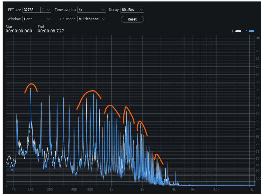
Figure 10: spectral analysis of a 50 Hz piano sound, with characteristic formants clearly visible
